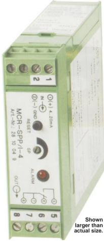
The MCR-SPP is a primary or redundant industrial process control alarm. The MCR-SPP module features a loop powered threshold monitoring circuit with a bi-stable relay, LED indication of relay status, configurable hysteresis function and relay action. Setting of the threshold is accomplished by a 20-turn potentiometer, while the configurable functions are set by movable jumper settings.
